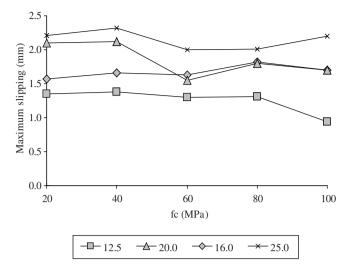
Figure 6. Maximum slipping vs. strength of concrete.
