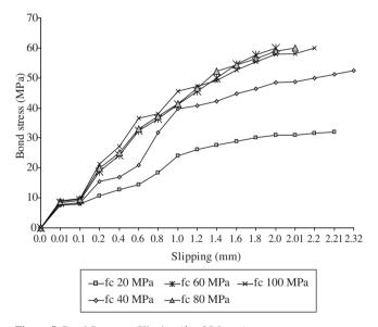
**Figure 5.** Bond Stress vs. Slipping ( $\phi = 25.0 \text{ mm}$ ).
