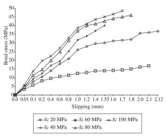
**Figure 4.** Bond Stress vs. Slipping ( $\phi = 20.0 \text{ mm}$ ).
